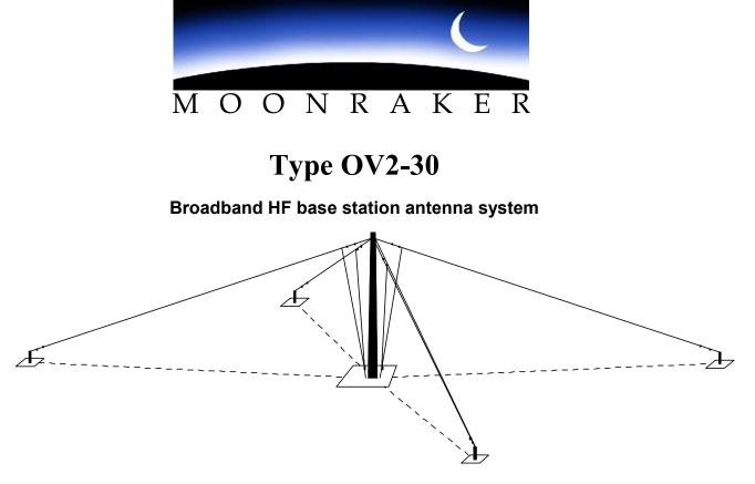
The Type OV2-30 is an omnidirectional wire antenna system that covers a base area of approximately 7200 sq m. ( $85 \times 85$ ) with a central mast approximately 20 metres tall. It has a continuous power supply capability of up to 1kW in the frequency range 2 to 30 MHz. It is designed to provide efficient and reliable communications in the professional/military services and is normally custom configured to suit site and communications parameters.
