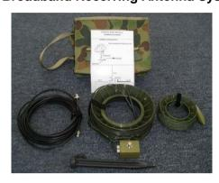
The Moonraker HF MRA RXMP is designed to provide reception from 2-30 MHz in the field. The system features a matching transformer with coaxial connector and uses two fast deployment reels, one for the antenna and the other for the counterpoise.
