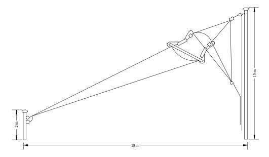
The semi-delta antenna system is designed for base station use by military, professional and commercial users of the HF band where a broadband system is required. Being simple to erect it exhibits an omnidirectional high angle radiation pattern for communications up to 1700 kilometres, dependent upon ionospheric conditions.
