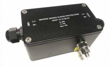
The protectors should be fitted at the point of entry of the cables to the interior of the vessel. Connection in the type DC or type AC cable is via sealed cable glands and internal screw terminals. The lid of the housing is fitted with an O ring seal. The housing is mounted via two bolts (not supplied) through the mounting plate.
