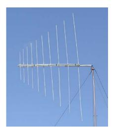
The BLP50-200 is a compact antenna, designed to provide wideband directional transmission of radio signals in the VHF band.
