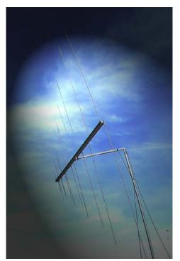
The BLP30-200 is designed to provide wideband directional transmission of radio signals from 30 to 200 MHz.
