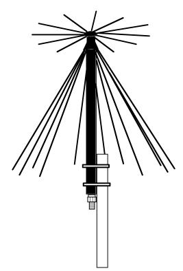
The BDA500 is designed to provide wideband omnidirectional communications over the 380-550 MHz military aviation band, providing excellent ground to ground as well as ground / sea to air communications.
